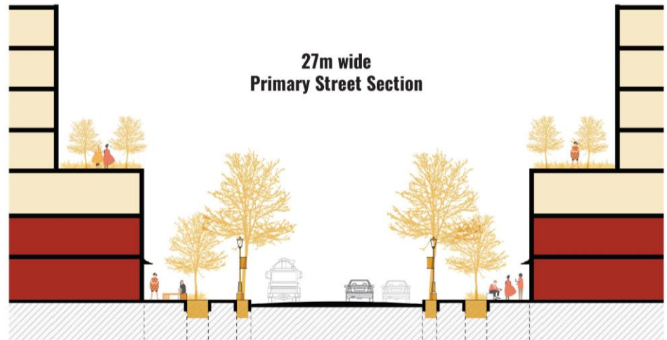
27m wide Primary Street Section Mixed Use Block Walk 3m Cycle 2m Carriageway 12m Cycle 2m Walk 3m Mixed Use Block STREET SECTION CC'
