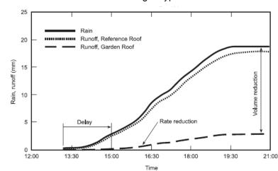
Figure 7-6 Cumulative Rain and Runoff during a Typical Rain Event
