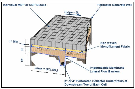
Figure 5-20 Grading of Permeable Pavement Structure
