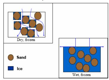
Figure 4-7 Ice Formation in Infiltration Systems
