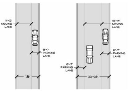
Left: 18-ft (5.5 m) street with parking on one side. Right: 22 (6.7 m) to 26-ft (7.9 m) street with parking on both sides. Source: PSAT, 2005, adapted from NHAB.
