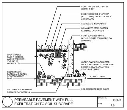
Figure 5-10 Permeable Pavement with Full Exfiltration to Soil Subgrade
