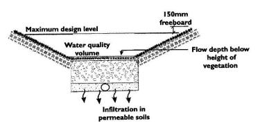
Figure 2-1 Typical Bioswale
