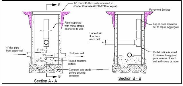
Figure 5-22 Example of Control Structure – UD&FCD
