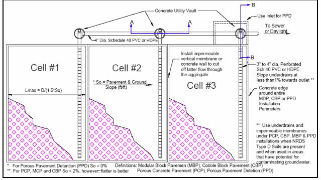
Figure 5-21 Subdrain System Layout for Permeable Pavement
