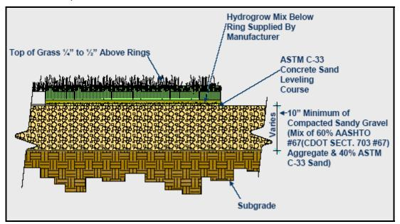
Figure 5-17 Example Cross-Section of Grass Pave Section
