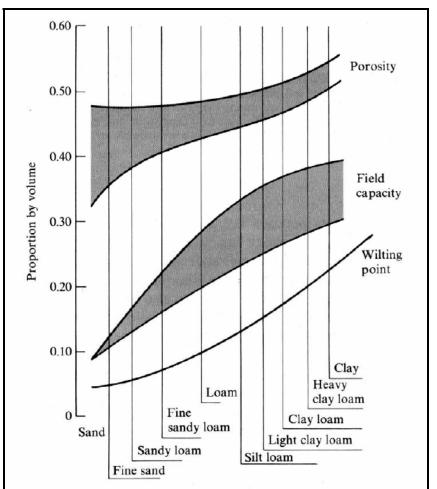
Figure 2-2 Soil Moisture Retention Capability as function of Soil Texture
