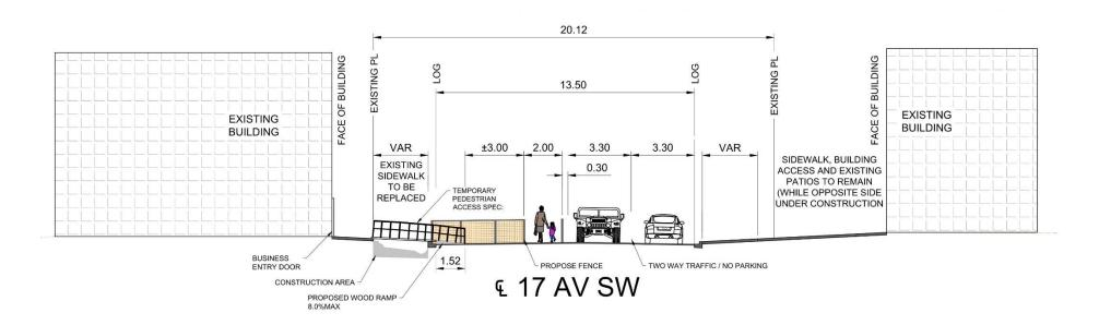
TYPICAL ROAD CROSS SECTION DURING CONSTRUCTION
