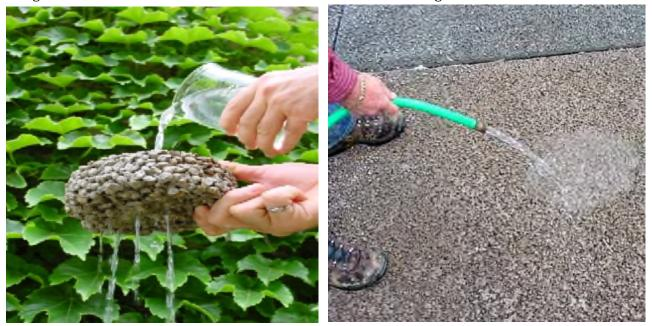
Figure 5: Pervious Concrete
