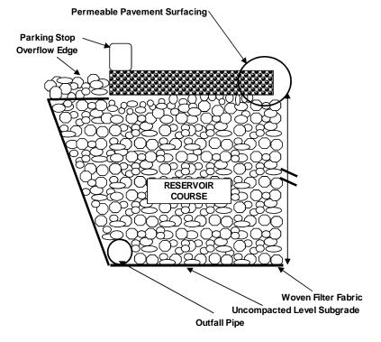
Figure 2: Typical Partial infiltration Porous Pavement Section with Subdrain System
