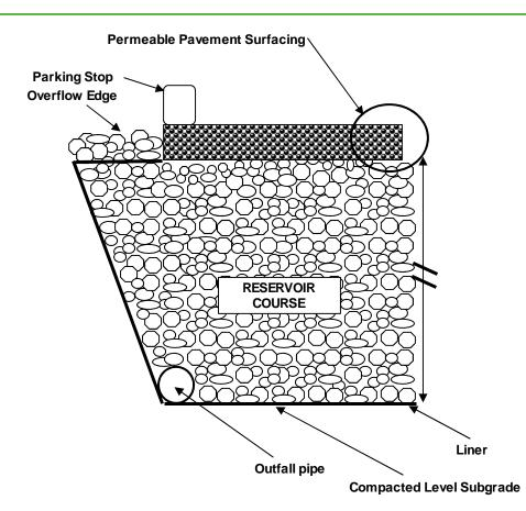
Figure 3: Typical No Infiltration Porous Pavement Section with Subdrain System
