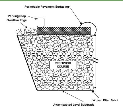
Figure 1: Typical Porous Pavement Section Infiltrating to Subgrade
