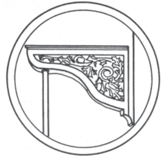
Handcrafted brackets were used to support the balconies. The columns were added later.
