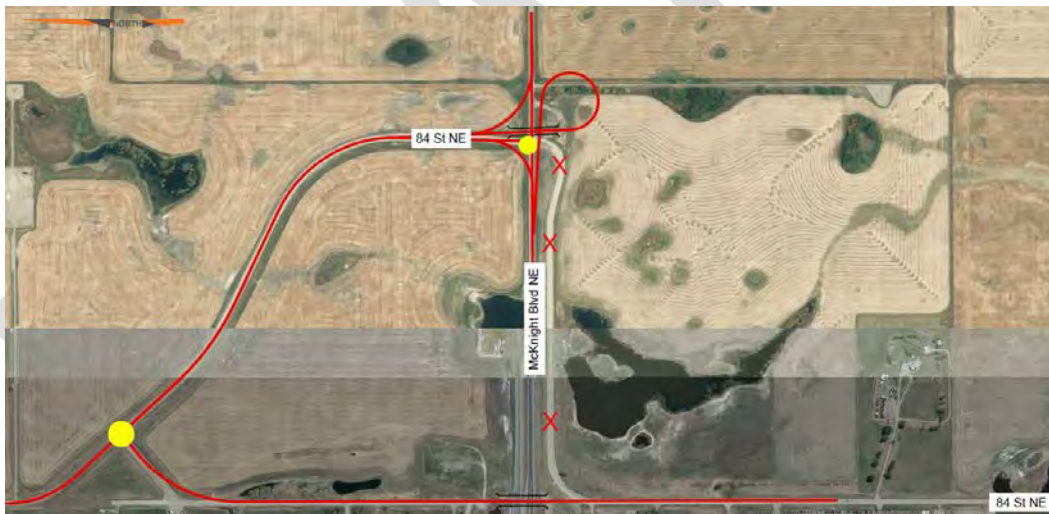
Figure 19 – McKnight Blvd Option 6 – 84 St Flyover with Left Turn Flyover
