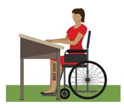
56. Where accessible picnic tables are provided, they are to be located adjacent to an accessible path of travel on a level, firm surface with a knee space at least 750 mm wide, 500 mm deep and 760 mm high.
