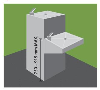
a) the alcove shall be not less than 850 mm wide, and b) the fountain shall be wall-mounted with clearance beneath the drinking fountain in accordance with the dimensions stated in the Alberta Building Code 2014 3.8.3.11.(1)(c).
