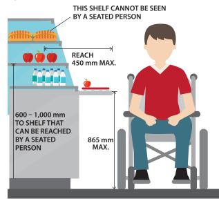
146. Counters shall contrast in colour/brightness from their surroundings, and surfaces shall have a non-glare finish. Explanation: Colour contrast and non-glare finishes can help people with vision loss locate and use counters
