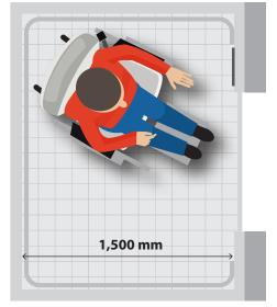
THERE SHALL BE ENOUGH SPACE IN AN ELEVATOR CAR TO ALLOW A PERSON IN A WHEELCHAIR TO TURN AROUND
