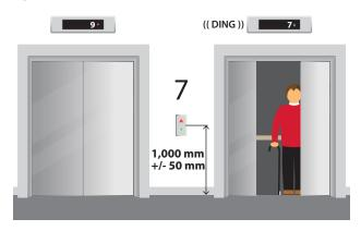
AN AUDIBLE SIGNAL SHALL INDICATE WHEN THE CAR HAS STOPPED AT EACH FLOOR
