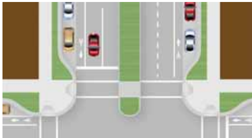
Figure 3.2-8: Integrating curb extensions and on-street parking into the sidewalk corridor enhances pedestrian safety and the walking experience (Credit: Michele Weisbart).
