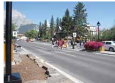
Figure 3.2-10: Raised median allows for pedestrian refuge (Banff Avenue, Banff, AB).
