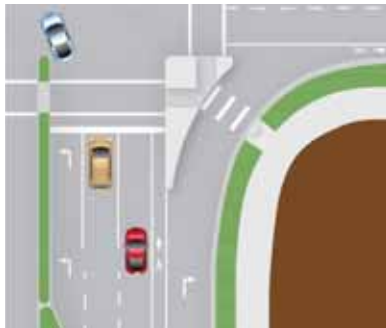
Figure 3.7-9: Traffic channelization is an effective mitigation strategy when intersection radii reduction is not an option (Credit: Michele Weisbart)
