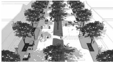
Figure 3.2-11: Angled median crossing (Credit: ite.org)
