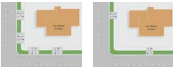
Figure 3.8-2, 3.8-3: Reconstructed corner with fewer, narrower driveways (Credit: Michele Weisbart)
