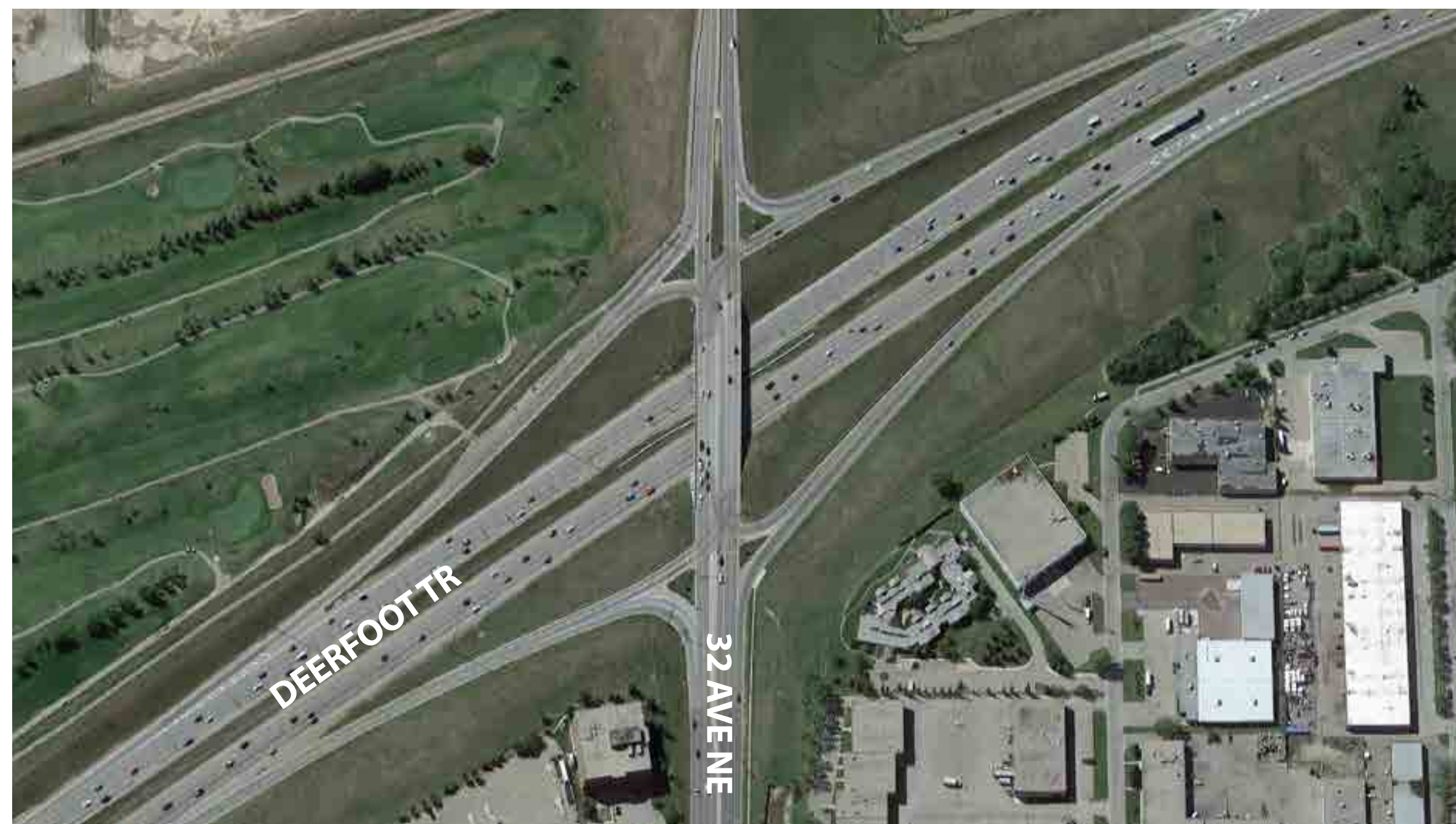
Caption: Deerfoot Trail at 32 Avenue N.E. is a local example of a conventional diamond interchange.
