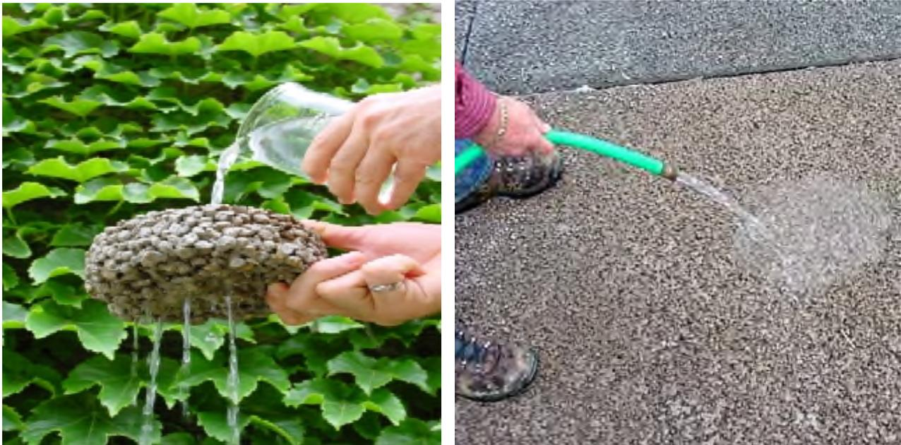
Figure 5: Pervious Concrete
