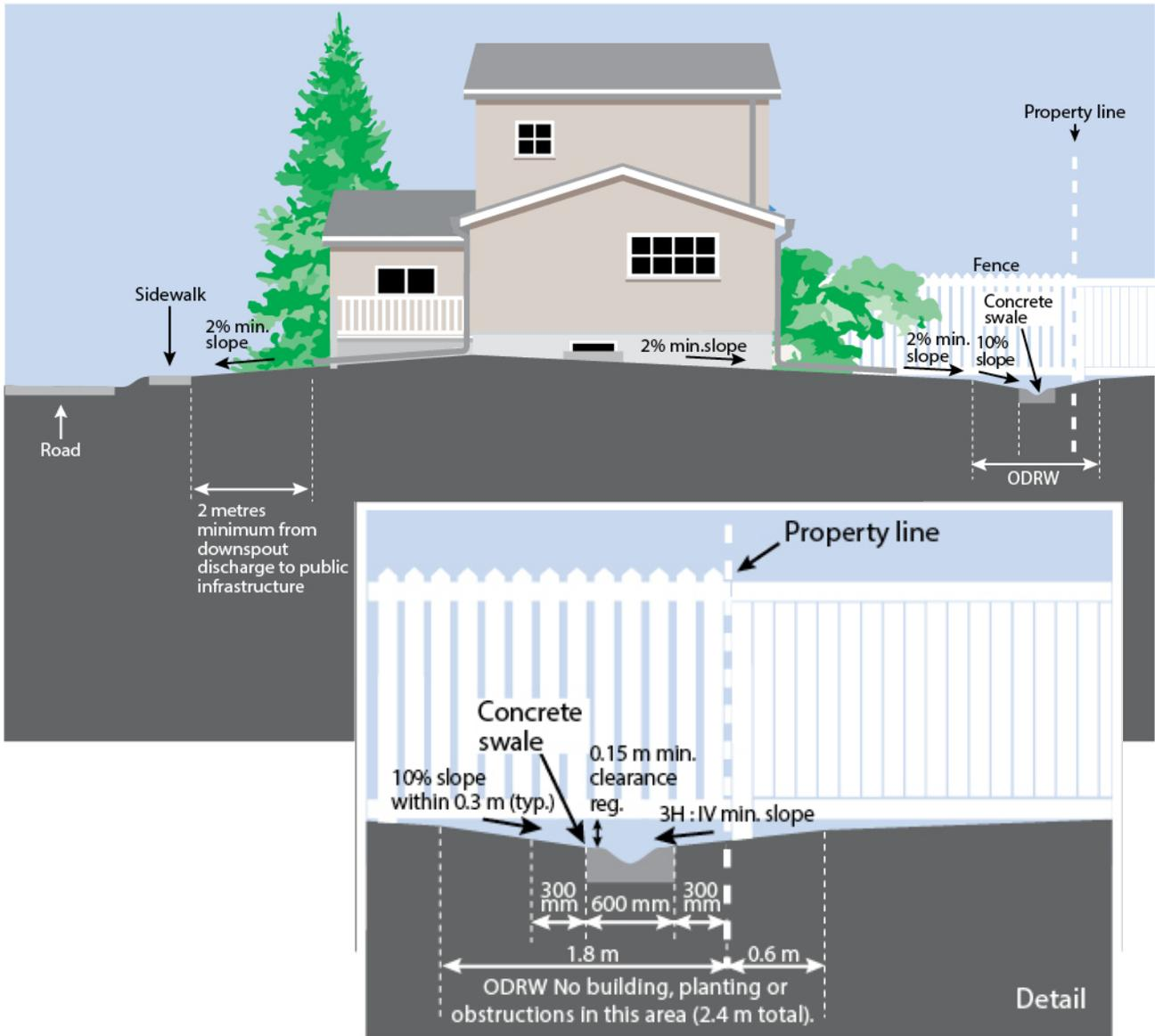
Figure 13 – Typical ODRW at Property Line / Fence. Source: The City of Calgary.
