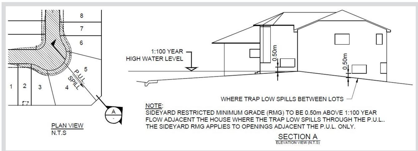
Figure 17 – Lot adjacent to a Trap Low with a Restricted Minimum Grade. Source: The City of Calgary Stormwater Management Guidelines.
