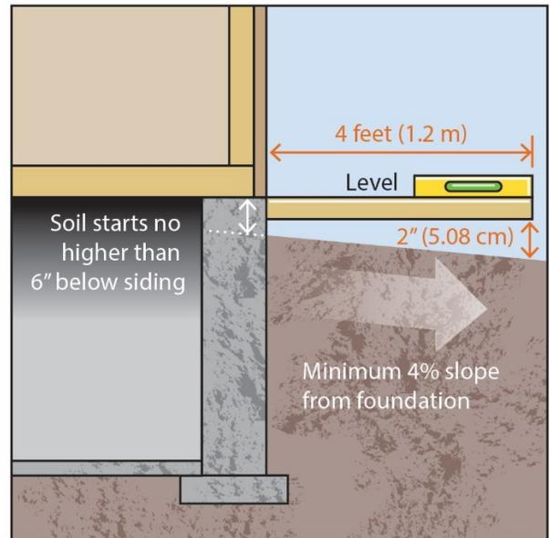
*How to Measure Slope. Minimum 4% Slope adjacent to foundations. Source: The City of Calgary*
