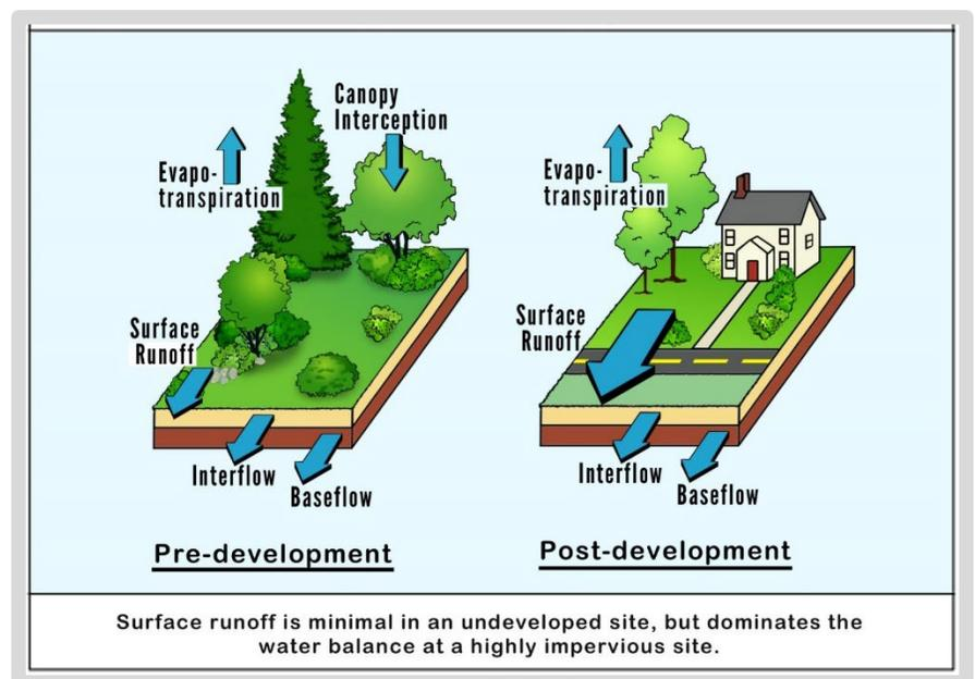
Figure 12 – Construction of Pervious Surfaces on a lot impacting stormwater run-off. Source: Schueler, 1987.
