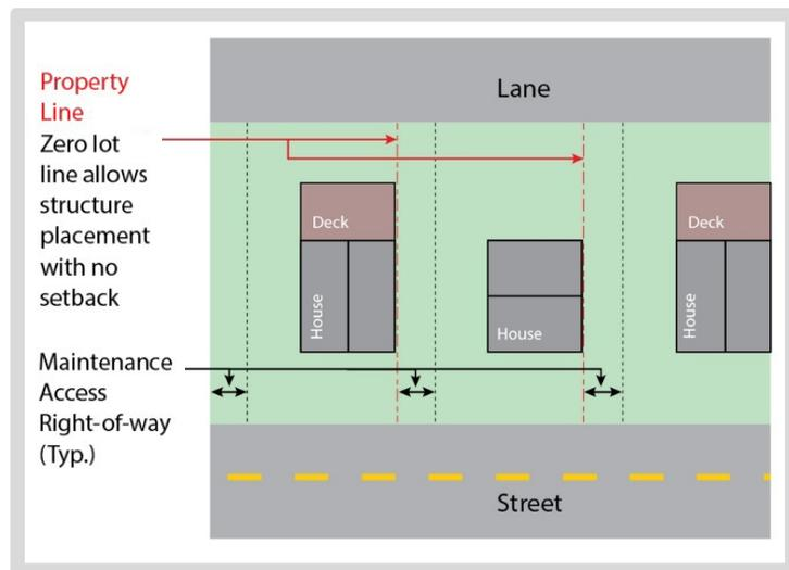
Figure 19 – Zero Lot Line with Maintenance Access Easement. Source: The City of Calgary.
