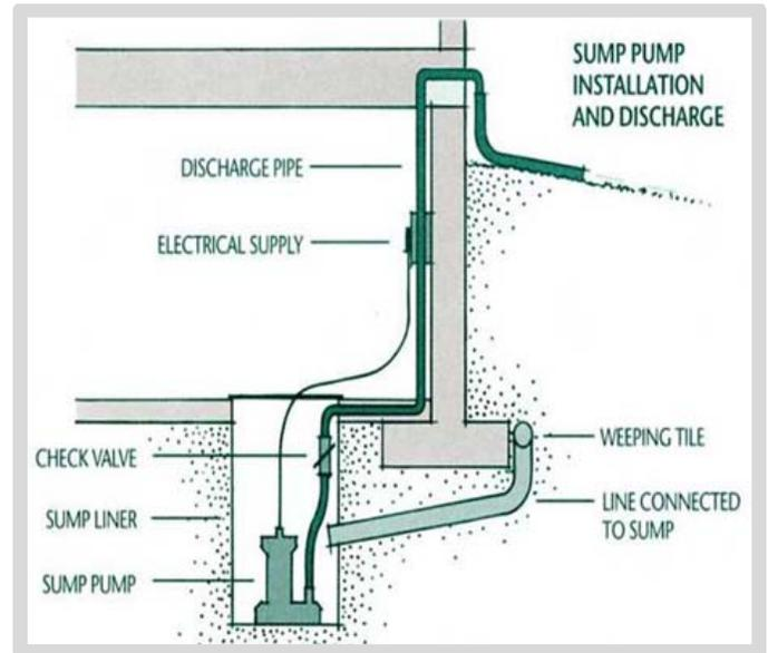
Figure 20 – Weeping Tile with Sump Pump.
