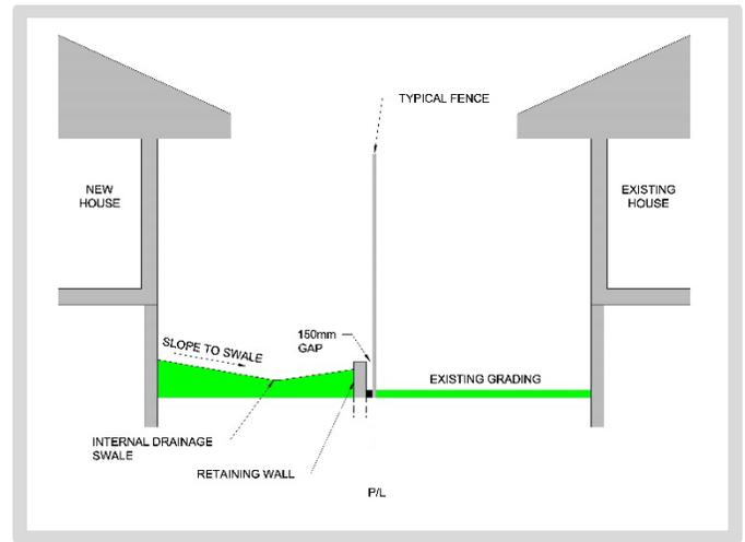
Figure 25 – Side Yard Swale and Low Retaining Wall. Source: The City of Calgary
