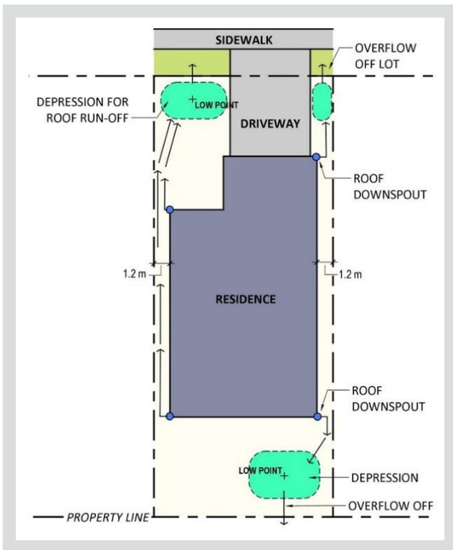
Figure 35 – Rain Garden Placement Example to Support Lot Drainage. Source: The City of Calgary
