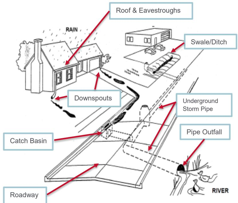
Figure 1 – Drainage System Components. Source: The City of Calgary Stormwater Management Design Manual.
