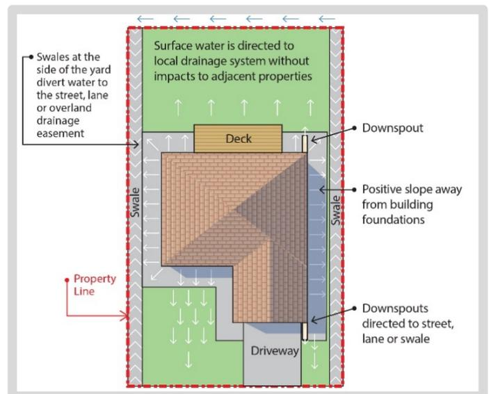
Figure 4 – Positive Lot Drainage. Source: The City of Calgary
