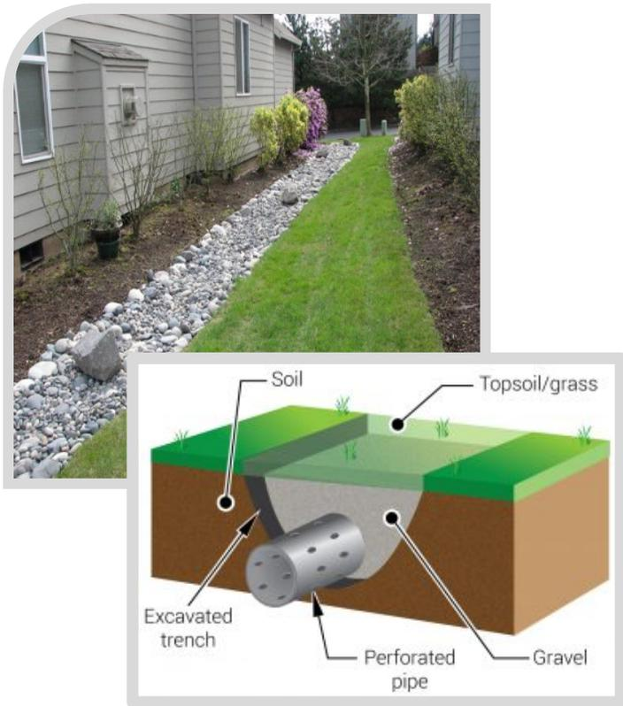
Figure 28 – French Drain Details. Sources: Neave Stormwater and engineeringclicks.com
