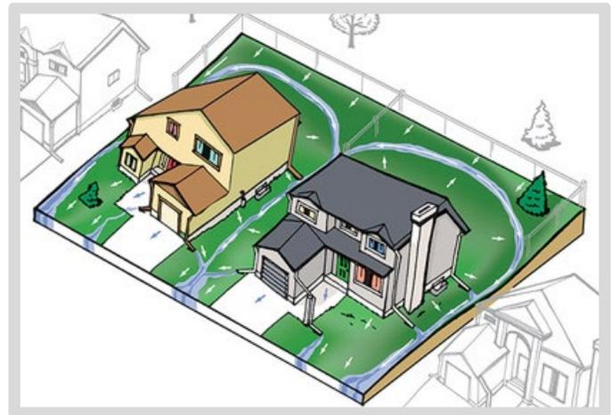
Figure 3 – Positive Lot Drainage to Swales. Source: The City of Edmonton Lot Grading Guidelines, April 2018
