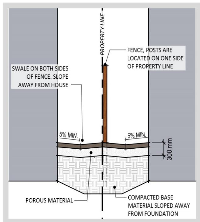
Figure 27 – Examples of Retaining Wall and Fence placement at Side Yard. Source: The City of Calgary.
