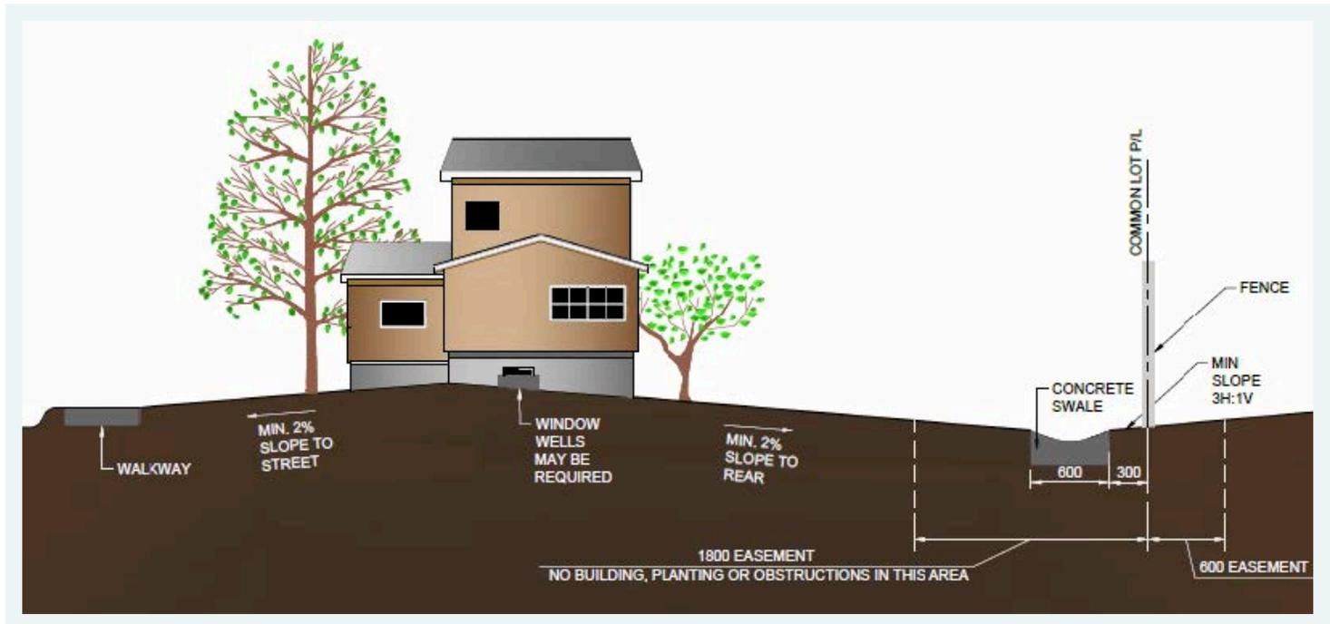
Figure 10 – Positive Lot Drainage with a Rear Yard Concrete Swale. Source: The City of Calgary
