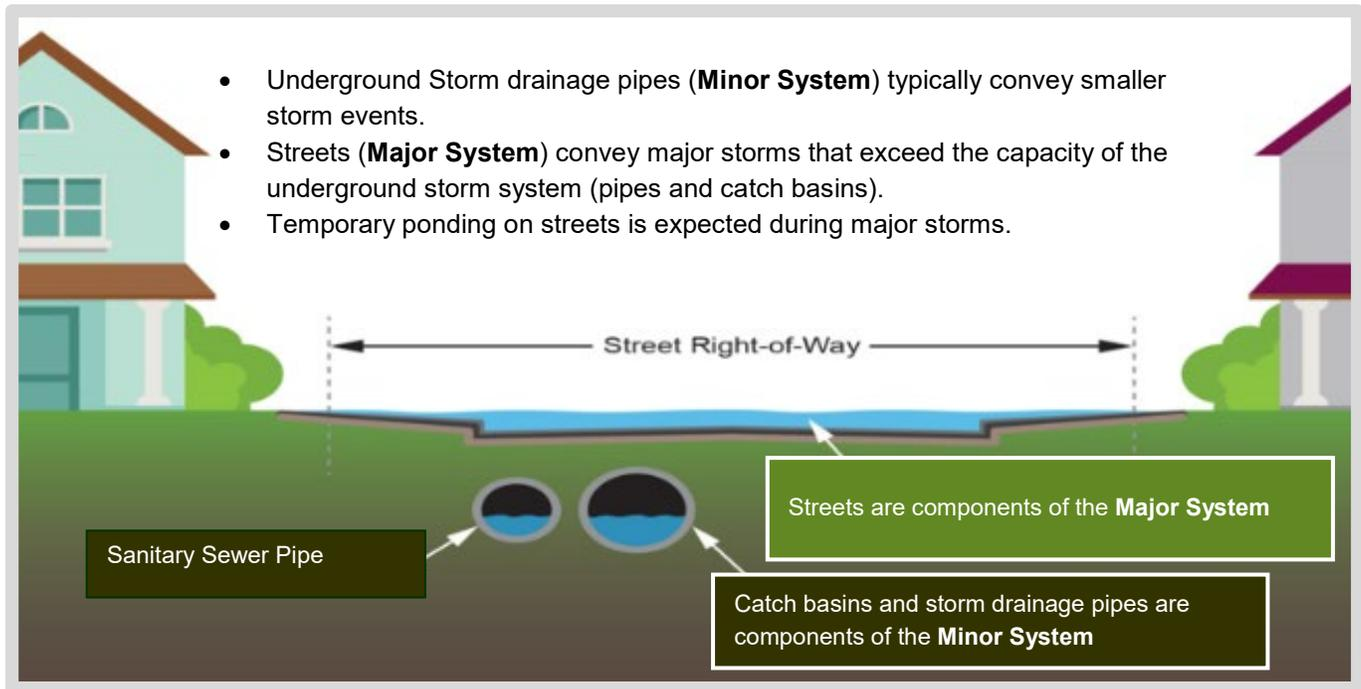
Figure 2 – Dual Drainage Concept. Source: Adapted from The City of Toronto.
