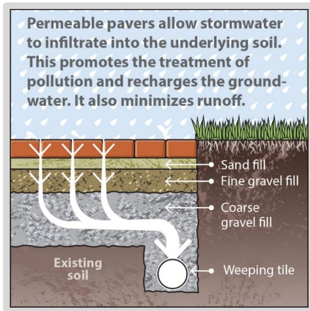
Figure 38 – Permeable Pavement Installation.
