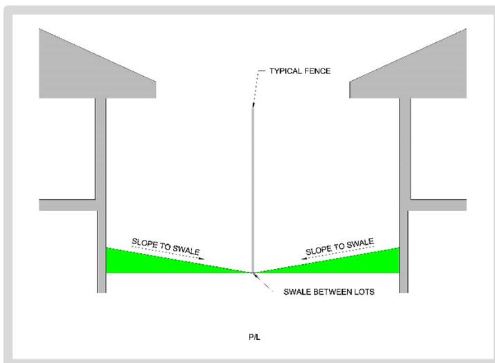
Figure 23 – Common (Shared) Side Yard Swale.
