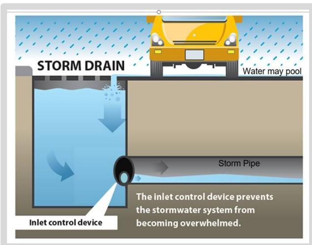
Figure 18 – Inlet control device in a catch basin to restrict flow. Source: The City of Calgary.
