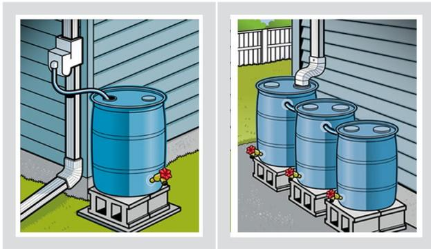
Figure 30 – Rain Barrel Placement to Capture Roof Drainage.
