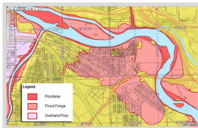
Figure 7 – City of Calgary Regulatory Flood Map identifying areas within the Floodway, Flood Fringe or Overland Flow Areas. Source: The City of Calgary Flood Information Website.
