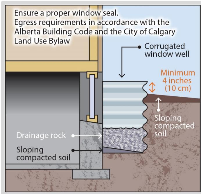
Figure 22 – Window Well grading. Source: The City of Calgary
