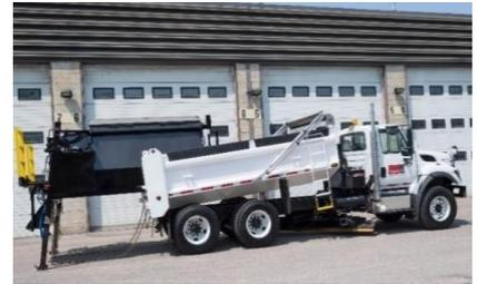
All three pieces of equipment are plug-'n-play using the same control system installed on the base dump truck. In less than 30 minutes, one operator can change the equipment and make the unit ready for the next application.
