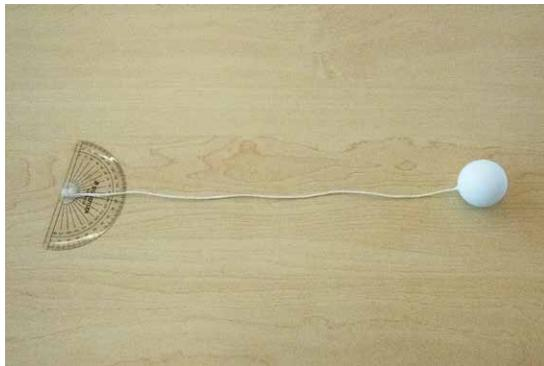
4. Place a drop of super glue in the middle of the flat edge of the protractor. Stick end of string to this glue. Let dry for at least 10 minutes.
