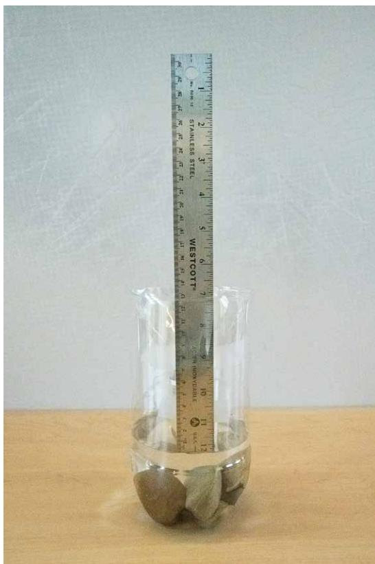
2. Place rocks in bottom to level surface and provide weight.
