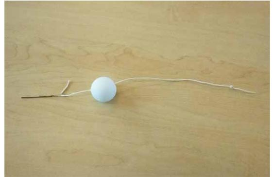
3. Puncture the ping-pong ball with the needle, pulling through the string and leaving the knot inside the ball. Remove the needle from the string.
