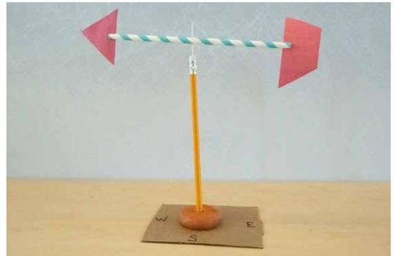
7. Place somewhere on a flat surface outside. Use the compass to orientate the weathervane so that North is facing true north.
