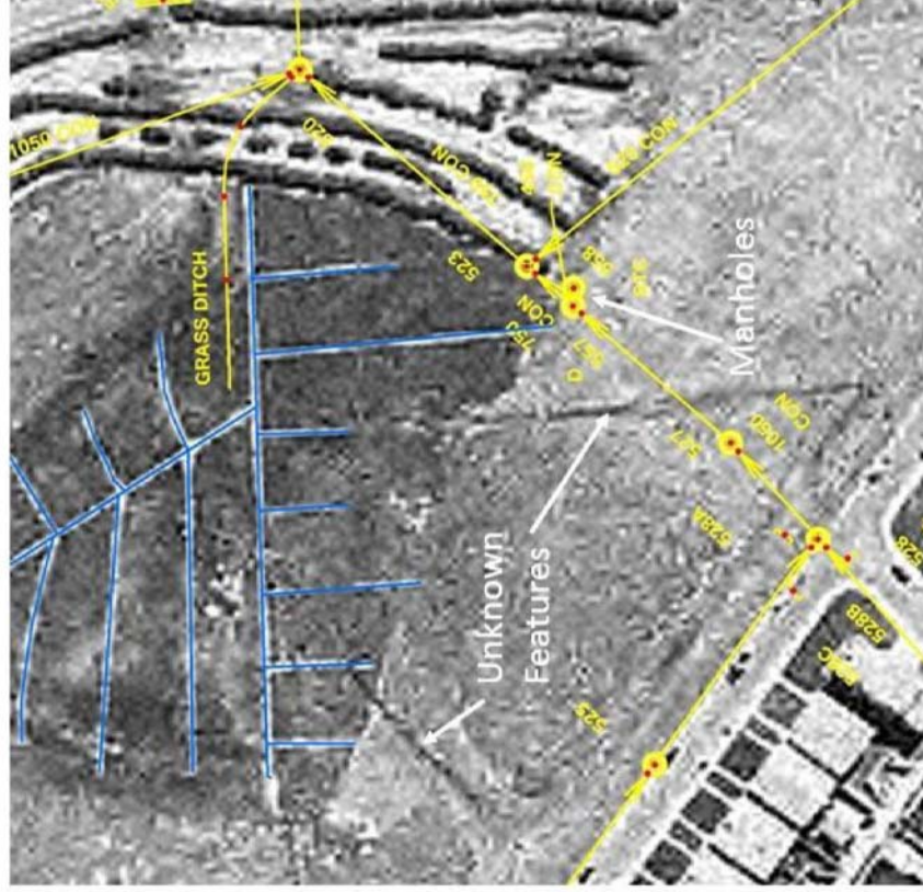
Left panel: Aerial photo of Canmore Park in 1966 showing the presence of tile drains in the wetland area. Right panel: a zoomed in view of the drains (highlighted in blue) in relation to stormwater infrastructure (yellow), note unknown features extending to the south and southwest.
