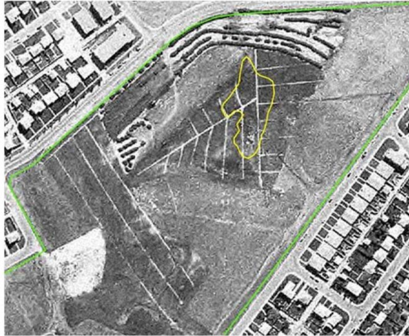
Left panel: Aerial photo of Canmore Park in 1966 showing the presence of tile drains in the wetland area. Right panel: a zoomed in view of the drains (highlighted in blue) in relation to stormwater infrastructure (yellow), note unknown features extending to the south and southwest.
