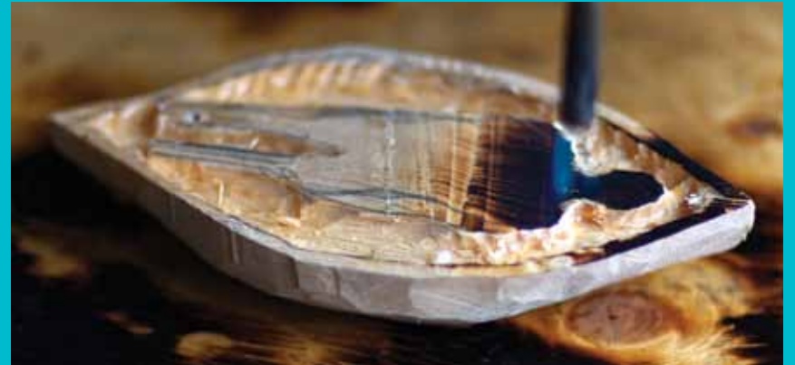
▲ The relief surface is charred with a propane torch.
