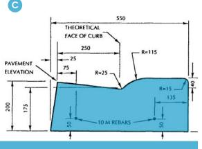
**C: Figure 6.3 Low Profile Rolled Curb Crossing** City of Calgary Standard Detail 454.1003.008B
