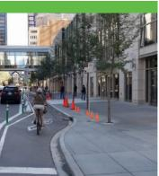
• Cycle Track: An enhanced bike lane, distinct from the sidewalk, that is separated by a physical barrier from moving and parked cars
