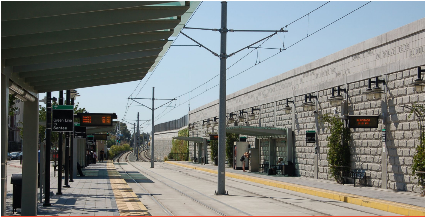
PL1 Pole: round/beveled galvanised steel poles- single use
