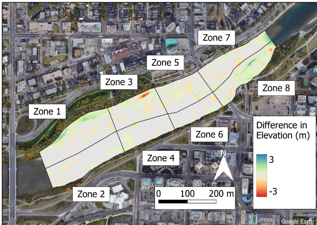
Figure 36. As-built initial bathymetry for CAL1 minus the target pre-flood bathymetry from Golder Associates (2011). Differences in elevation between -0.15 m and 0.15 m are shown in grey. Zone names conform to Table 10.
