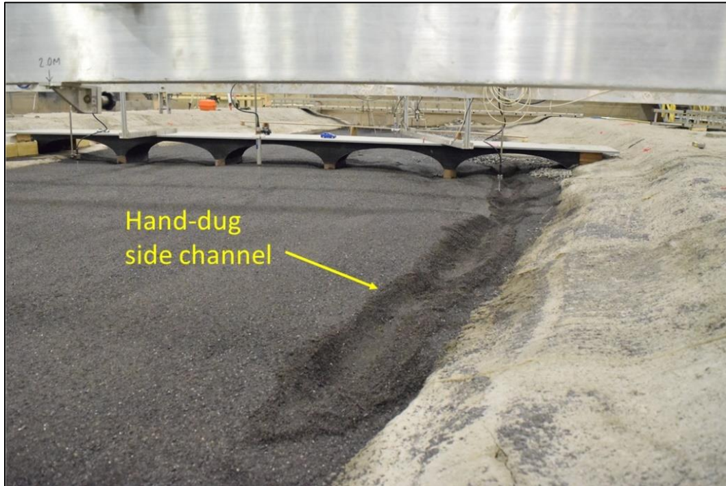
Figure 34. Bathymetry modification for the do-nothing test.
