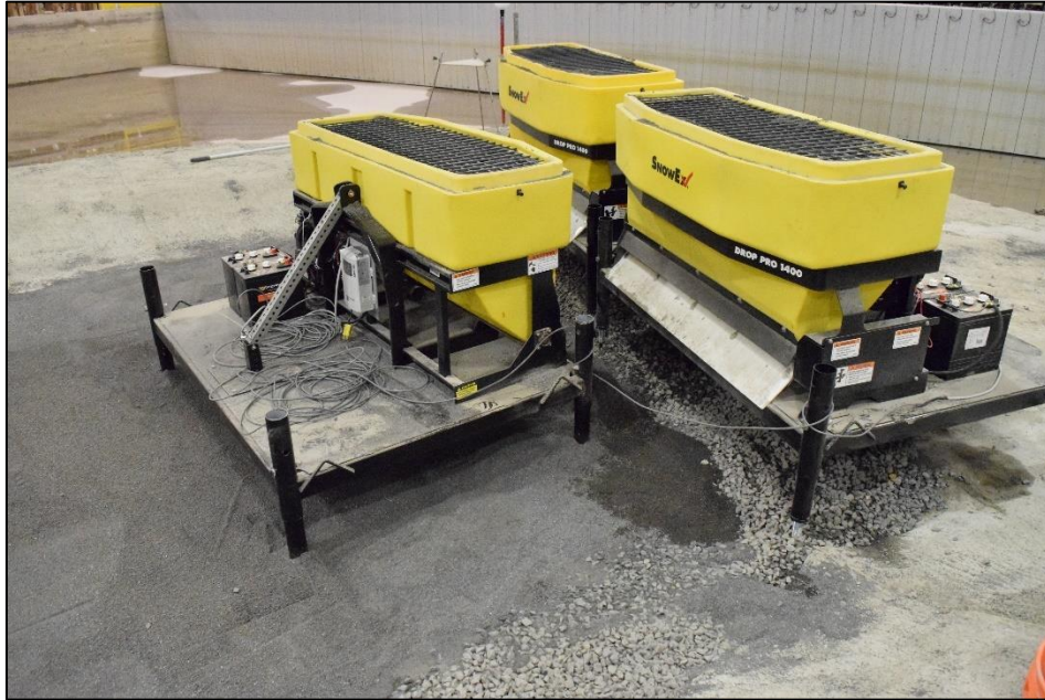
Figure 23 Sediment spreaders installed at the upstream boundary of the model.
