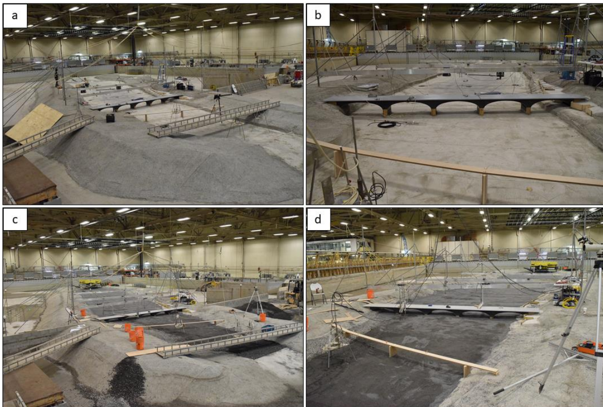
Figure 14. Photographs of the physical model after construction; a) and b) show the model without a mobile bed installed and c) and d) show the model with a mobile bed installed.
