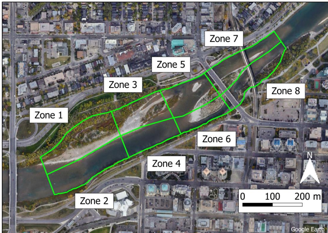
Figure 31. Zones used to assist with the interpretation of erosion and deposition, plotted over a post-flood satellite imagery basemap.
