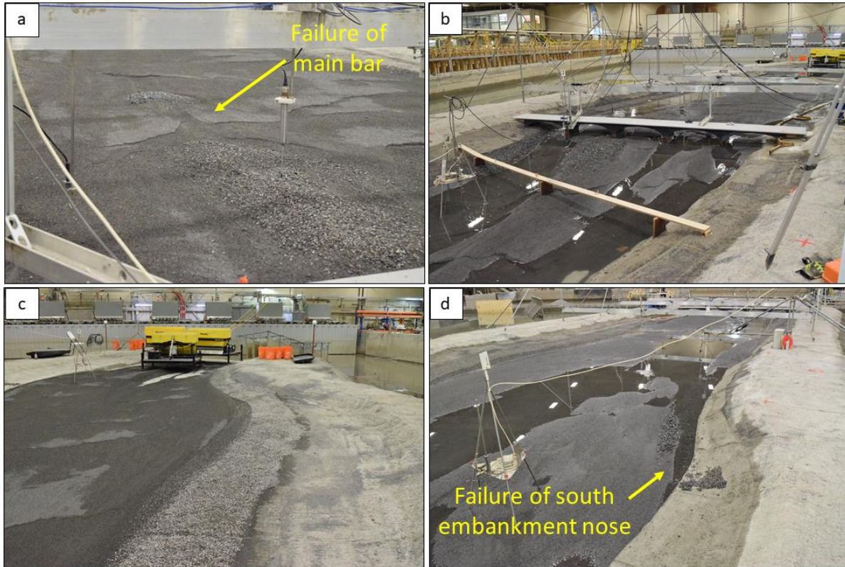
Figure 73. Photos of the model after TSA_2100; a) standing on Louise Bridge, looking upstream at the main bar, b) standing at the north side of the downstream boundary, looking upstream, c) standing at Poppy Plaza, looking upstream, d) standing near the south side of the upstream boundary, looking downstream.
