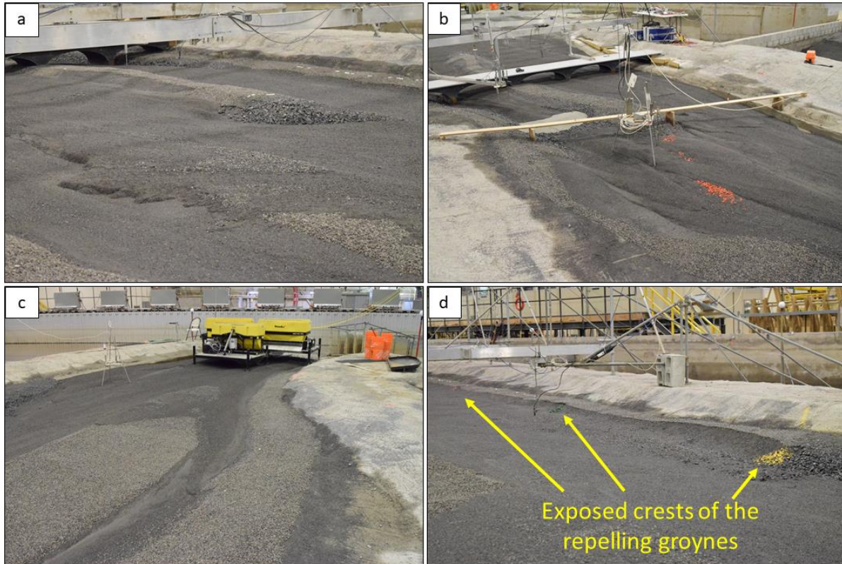
Figure 82. Photos of the model after TSB_850; a) standing at Poppy Plaza, looking across the channel and downstream at the main bar, b) standing at the south side of the downstream boundary, looking upstream, c) standing at Poppy Plaza, looking upstream, d) standing at the north side of the upstream boundary, looking at the south embankment.
