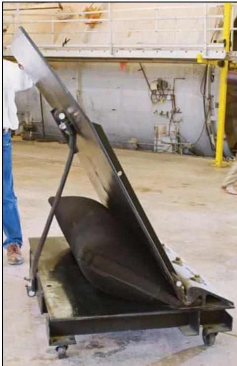
Figure 21: Example Obermeyer pneumatic gate not installed.
