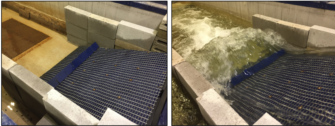
Figure 34: Wave forming with kicker at lower positions and with lower tailwater.
