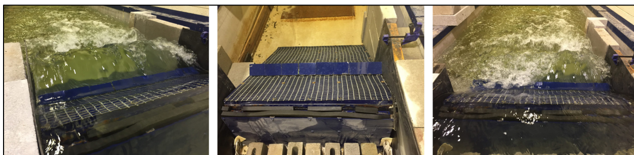
Figure 42: Physical modelling of sidewall impacts on wave formation. Left image shows walls above tailwater. Middle and right images show wall below tailwater. 17
