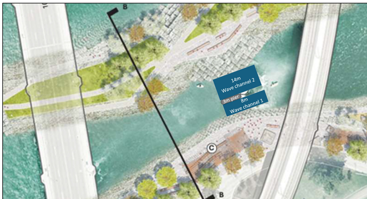
Figure 11: Adjustable wave structure channel and pier layout.
