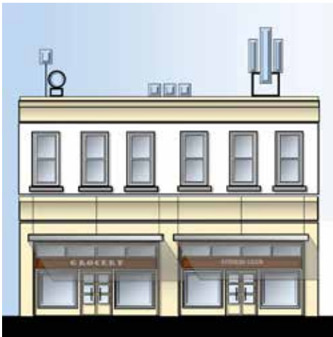
Films applied to antennas reflect the sky and minimize visibility from a distance.
