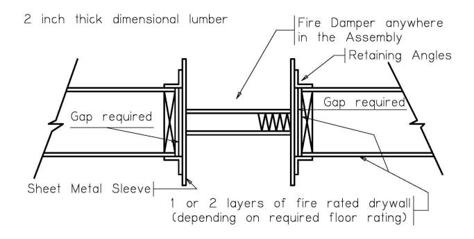
It has been queried whether the detail below is also acceptable, since doubts were expressed about the ability of I-joists to support the drywall and the damper in a fire situation as well as sawn lumber. (The only difference is that the sawn lumber sections have been replaced by engineered joists)
