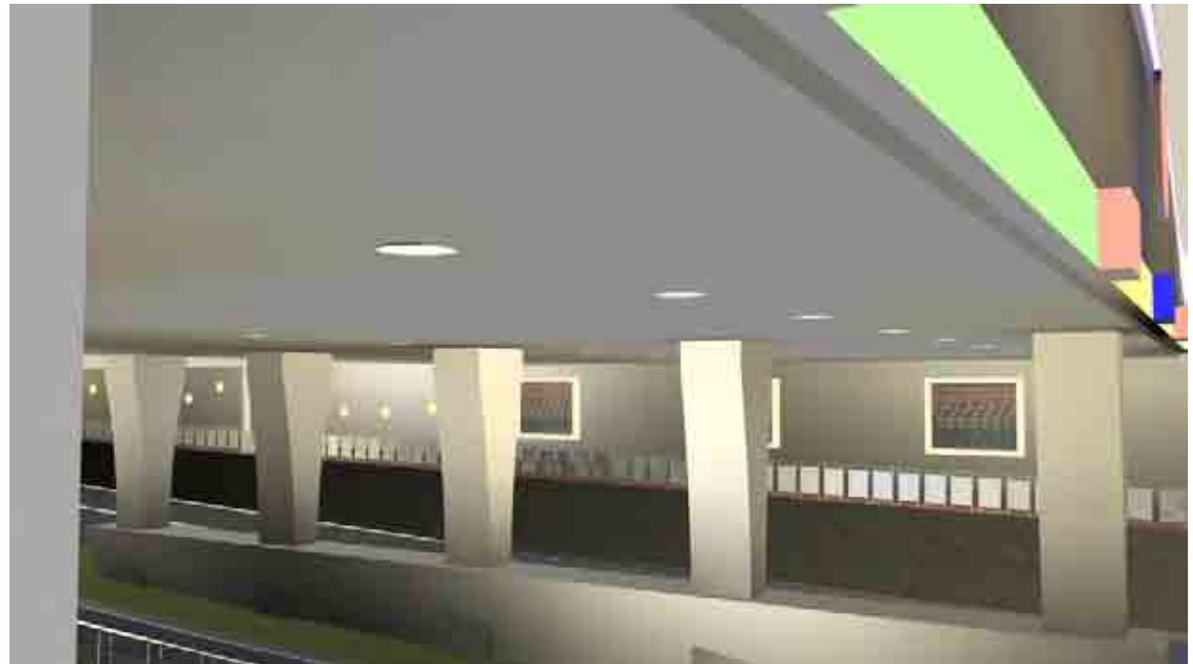
Image shows conceptual lighting underneath a rail bridge structure, and shows illumination of retaining walls along sidewalk and balustrade
