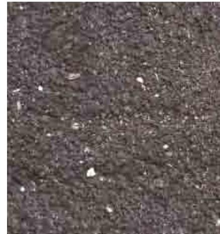
Permeable paving - porous asphalt
