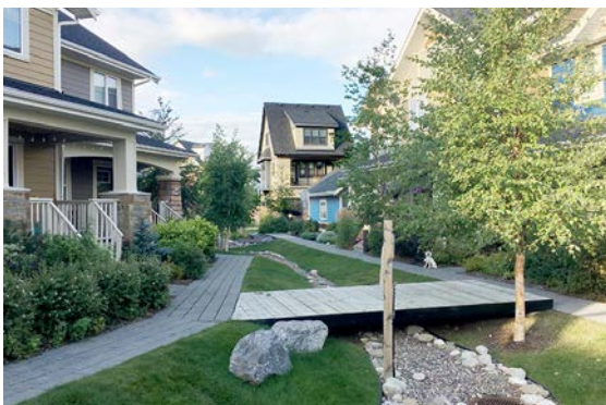
Photo: Residential landscaped area that incorporates features that collect, retain and absorb rain water.
