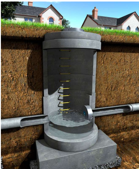
Figure 3.3: Manhole with a Vortex Flow Control Device 2
