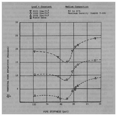
Figure 8 – Observed Vertical Ring Deflection in Buried Plastic Pipe as a Function of Pipe Stiffness<sup>14</sup>
