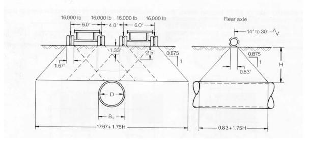
We'll continue to use an AASHTO HS 20 vehicle (depicted above in Imperial units), which has a total axle load of 142.34 kN (32,000 lbf) per truck for a total load of 284.69 kN (64,000 lbf).
