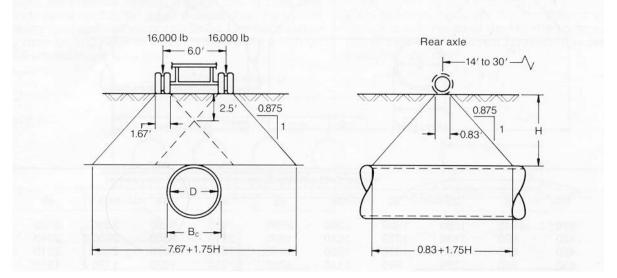
We'll use an AASHTO HS 20 vehicle (depicted above in Imperial units), which has a total axle load of 142.34 kN (32,000 lbf).
