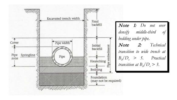
Figure 10 - Narrow Unsupported Trench - Typical
