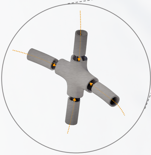
Bolted Sleeve Connection Detail at HSS Connection
