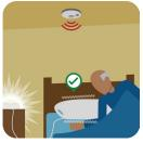
**Assistive alerting or signaling devices** work with existing standard smoke alarms. These devices are typically placed on a table beside a bed or seating area and look like an alarm clock.
