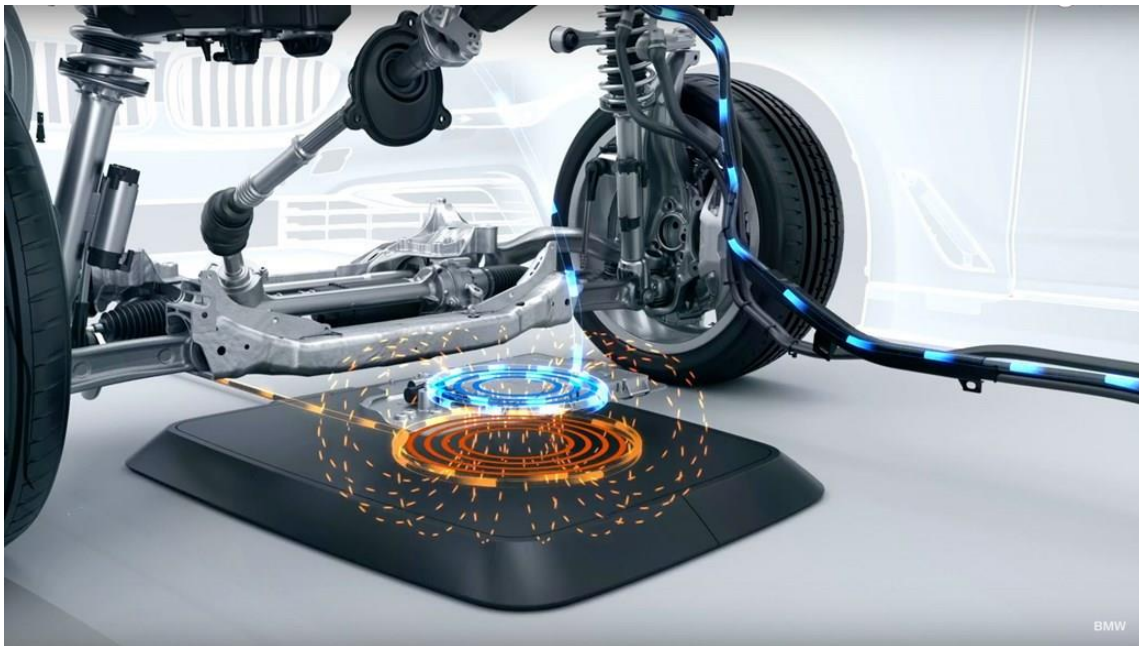
Figure 15: BMW EV Wireless charging mat and visualization of the magnetic field (dashed orange line), primary charging coil (orange) and secondary charging coil (blue) [143]
