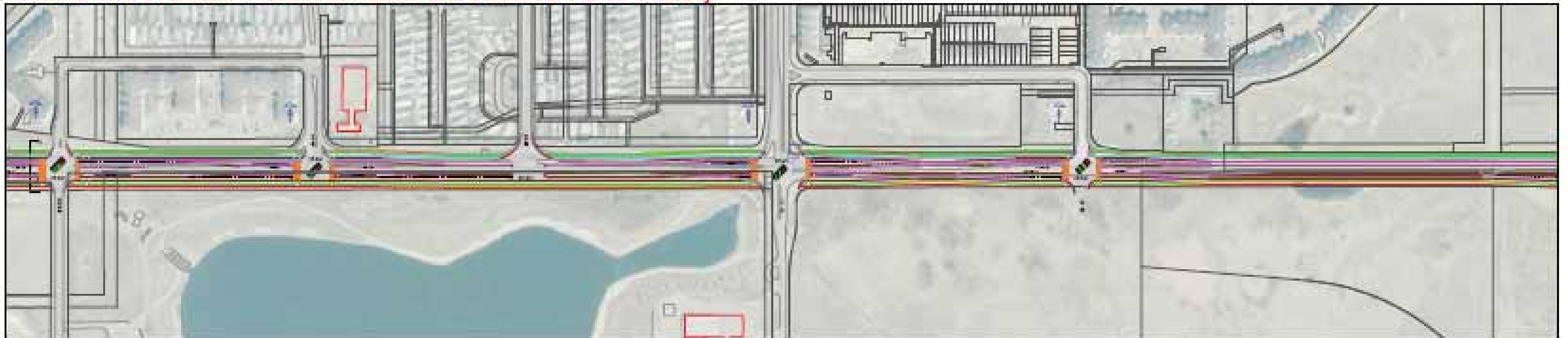
ALTERNATIVE 3 - Median Reserved Bus Lanes with 2 Lanes of Traffic - Parkway
