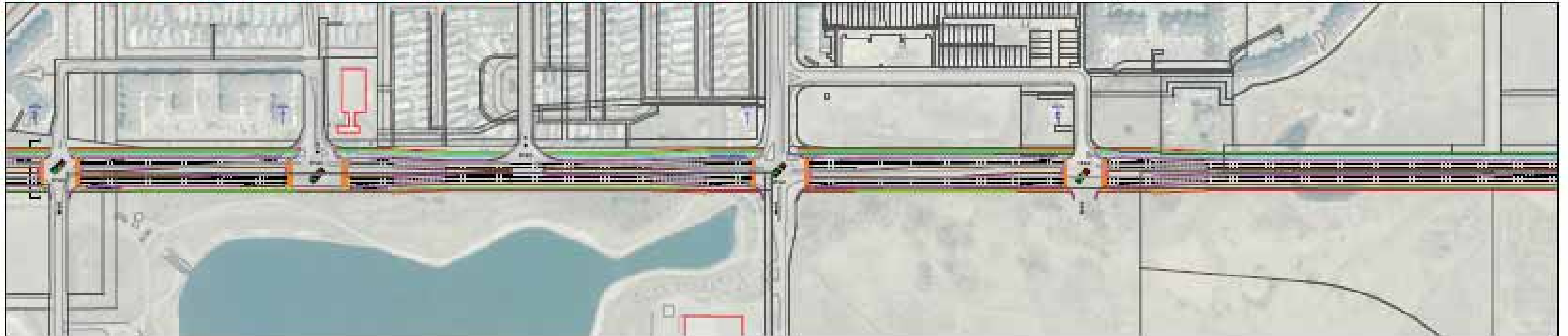
ALTERNATIVE 2 - Curbside Reserved Bus Lanes with 4 Lanes of Traffic - Parkway
