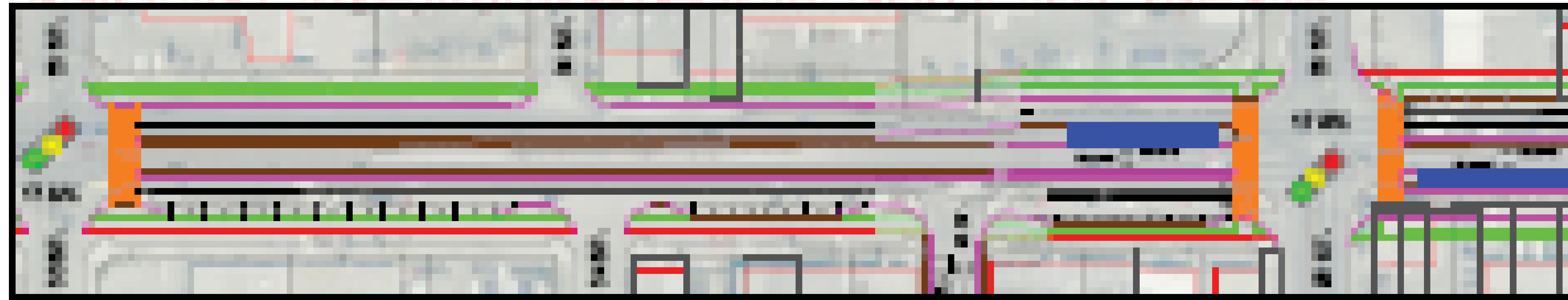
ALTERNATIVE 1 - Median Reserved Bus Lanes with 4 Lanes of Traffic - Urban Blvd.
