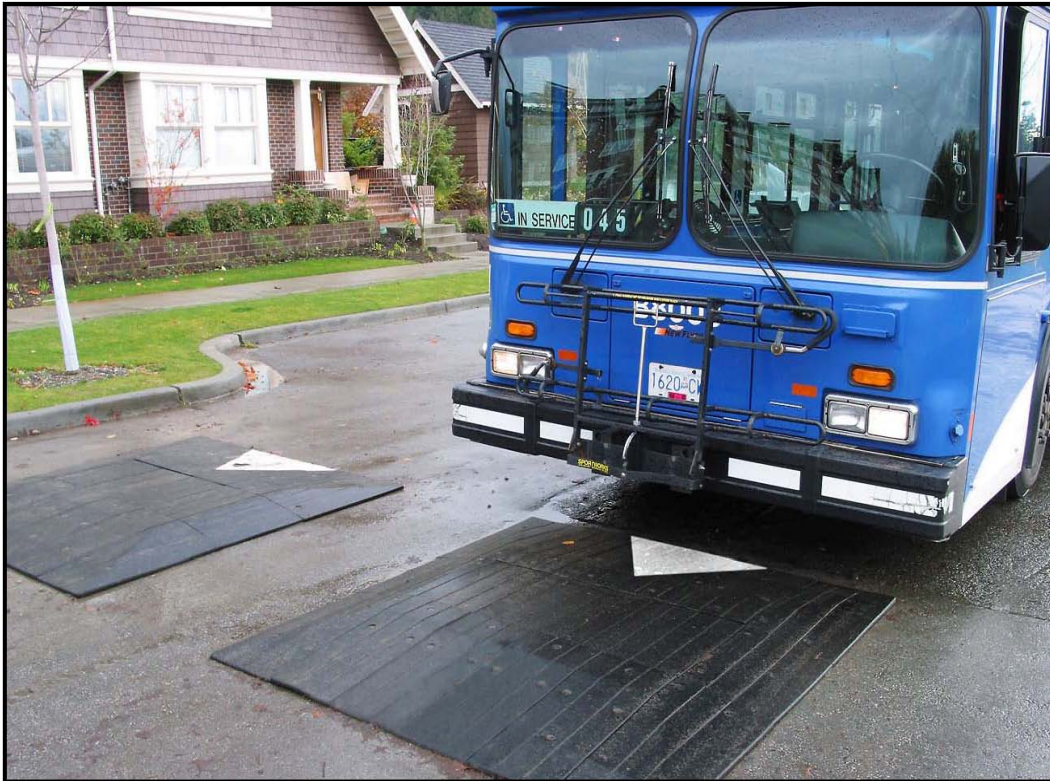
Figure 4.2 Speed Cushions with Transit Bus
