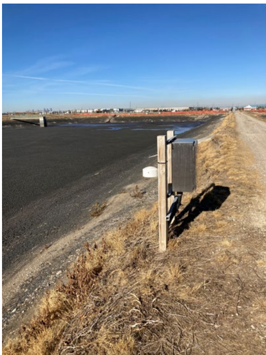
Photograph 4: Passive sampling with a diffusion tube (under white "mushroom cap") near the Biosolids Lagoons (looking northwest)
