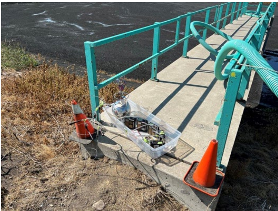
Photograph 2: Air Sampling near Biosolids Lagoons (Evacuated Canisters and Tubes with Pumps) Looking southwest.
