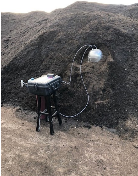
Photograph 3: Taking an odour sample using a flux chamber and Lung Sampler at the outdoor compost storage area – Looking south.
