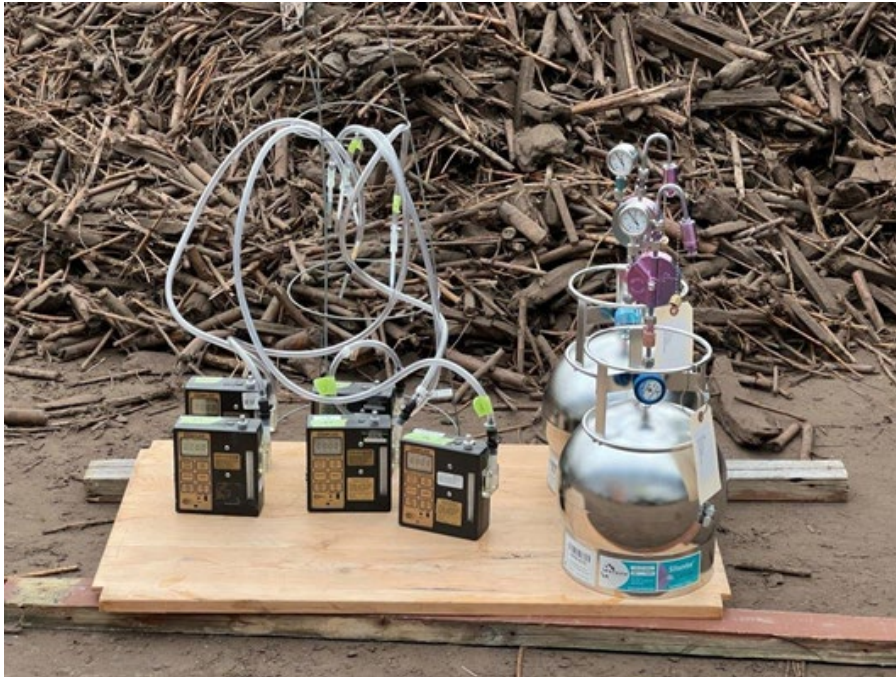
Photograph 1: Air Sampling inside Biofilter Building for the purposes of chemical speciation.
