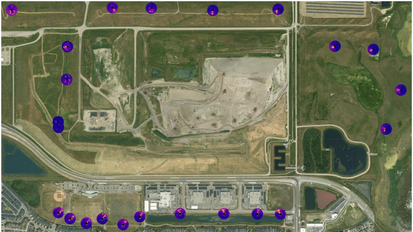
Figure 29. Aerial View of the Shepard Landfill and New Brighton Athletic Park with CH 4 Radial Surfaces at Each Inlet Location
