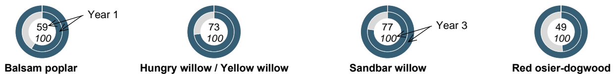
Figure 3-1: Year 1 (inner doughnut) and Year 3 (outer doughnut) Post-Construction Survival (%) of Common Live Cutting Species Used in Bioengineering Projects in Calgary (2018 and 2019 data)
