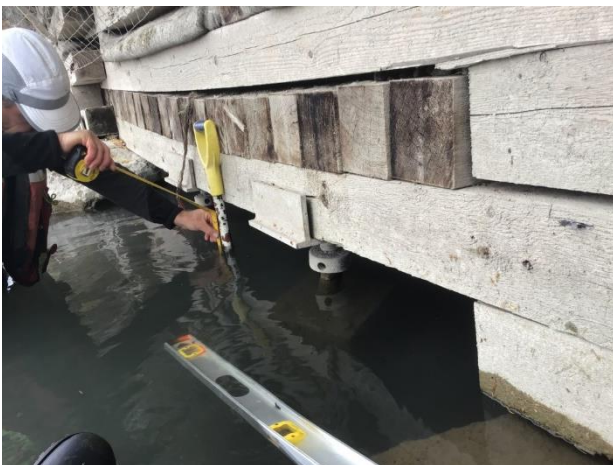
Photo E-11: Site 1 measuring sediment deposition in the fish shelters
