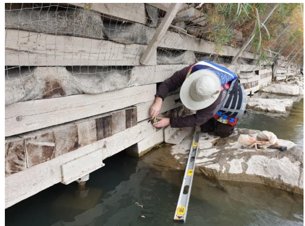
Photo E-12: Site 1 setting up spanning timber member deflection measurement points
