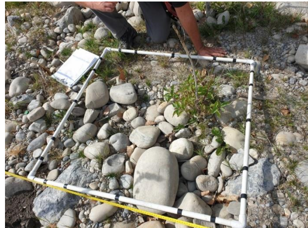
Photo E-18: Site 1 vegetated riprap with rooted long cuttings quadrat assessment
