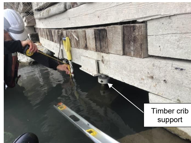
Photo 5-6: Measuring sediment depth in fish shelters and timber crib wall supports (September 25, 2020)
