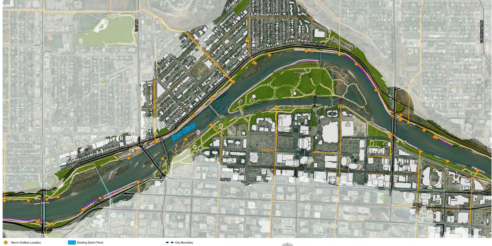
Stormwater Lift Station Storm Main (> 900mm diameter) Sanitary Main (>600mm diameter) Water Main (>400mm diameter) Pipeline River Crossing Locations
