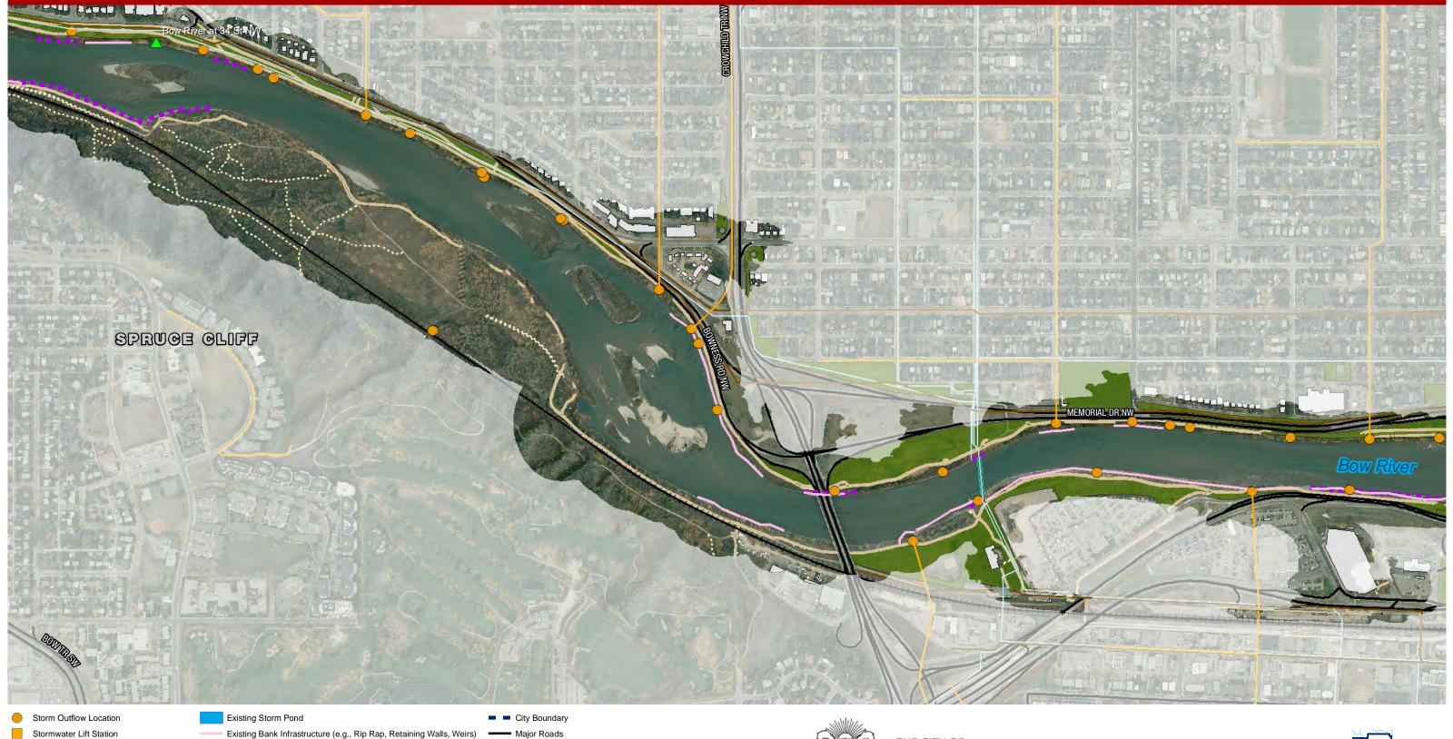
Stormwater Lift Station Storm Main (> 900mm diameter) Sanitary Main (>600mm diameter) Water Main (>400mm diameter) Pipeline River Crossing Locations Water / Waste Water Treatment Plants
