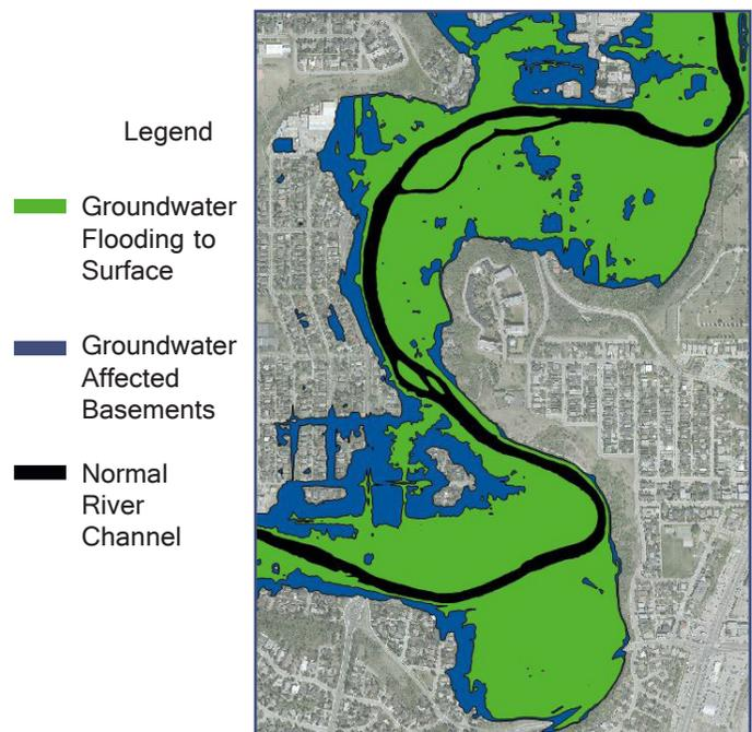
Figure 5 - Groundwater Inundation Mapping Example
