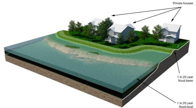
Figure 28 - Dyke Barrier
