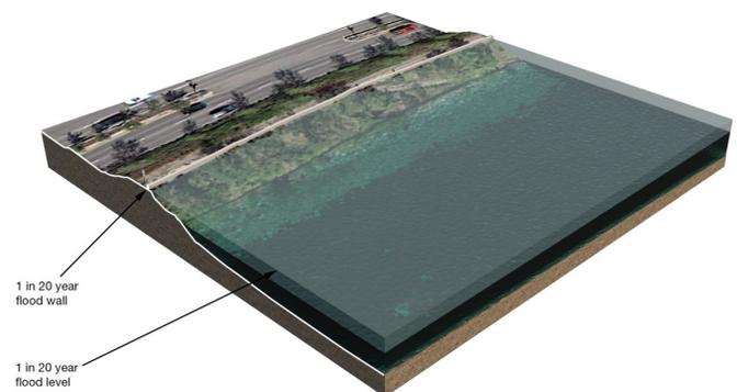
Figure 25 - Concrete Wall on Existing Barrier
