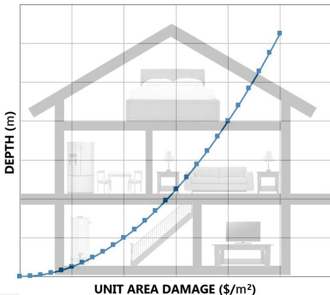
Figure 9 - Example Depth Damage Curve
