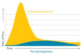
Figure 4: Changed hydrology due to urbanization
