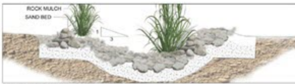
DETAIL 1 : BIOSWALE TYPICAL DETAIL
