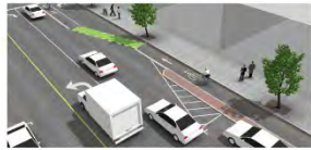
Unprotected bicycle lane through right-turn transitional zone
