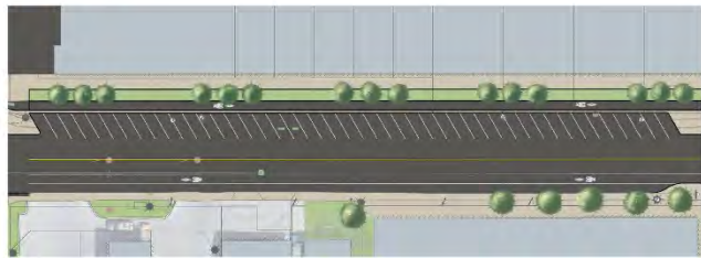
Sidewalk and landscaping closest to the building face with a bike lane protected by angled parking on Bowness Road N.W.
