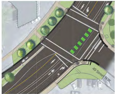
Unprotected bicycle lane through right-turn transitional zone
